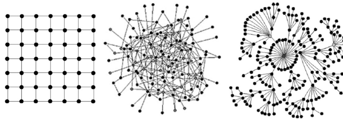
Figure 7.5. Three different kinds of network: a regular lattice or ordered grid (on the left), a random network (in the middle) and scale-free network (on the right).
